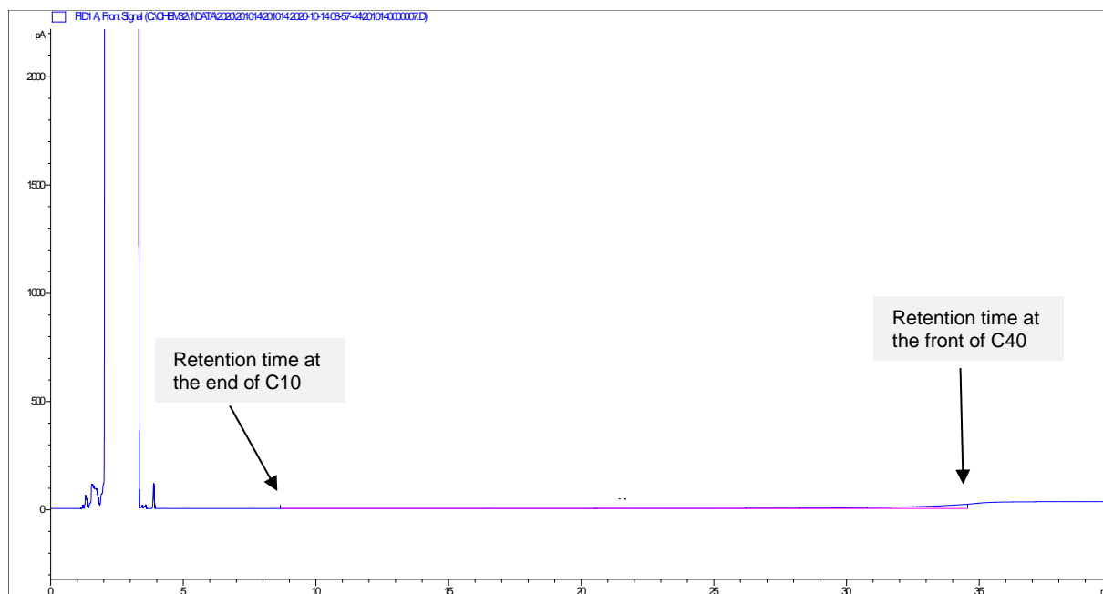
Fig. 5: Integrated GC-FID chromatogram of n-heptane (blank, pure solvent used to prepare BAM-K010g dilutions) between the retention times of C 10 and C 40 (analyzed on a BPX-5 column)
