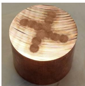
Fig. 2: Measurement scheme for radial homogeneity testing
