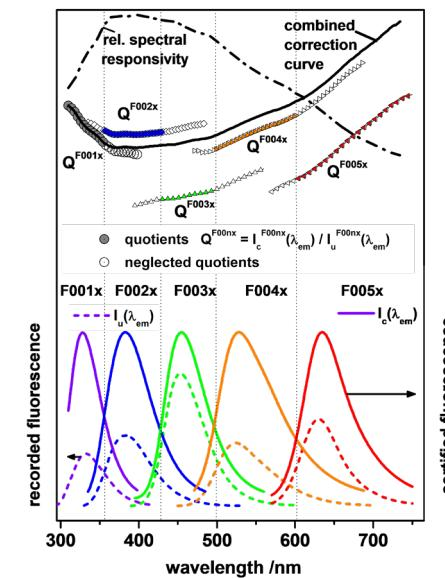
Bottom: Certified normalized corrected emission spectra ( $I_c(I_{em})$ ) of the kit components and uncorrected, i.e., instrument-dependent emission spectra ( $I_u(I_{em})$ ), measured with the instrument to be calibrated.
