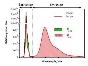
Fig. 2 Scheme of the determination of the relative photon flux emitted from the sample (red area) and the relative absorbed photon flux (green area) measured with an integrating sphere setup.
