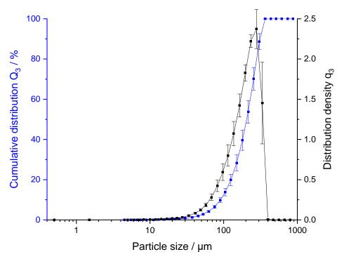
Average value distribution of 10 measurements by laser diffraction under dry dispersion (HELOS/BR + RODOS/L + ASPIROS, Sympatec, Germany, ISO 13320:2009 certified).
