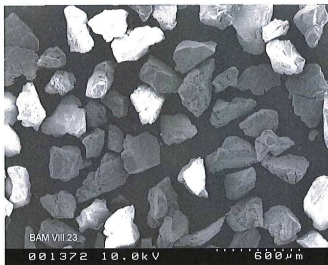
Figure 3: Scanning electron micrograph of \alpha -alumina
