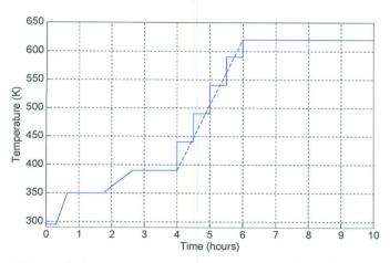
Figure 2: Recommended heating curve for the microporous material ERM<sup>®</sup>-FD107
