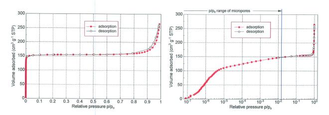
**Figure 1:** Linear and logarithmic plot of the nitrogen adsorption isotherm (non-certified) at 77.3 K and p/p₀-range for micropores (width ≤ 2 nm) according to the physical parameters applied in the Saito/Foley model with cylindrical pore geometry given on page 3.
