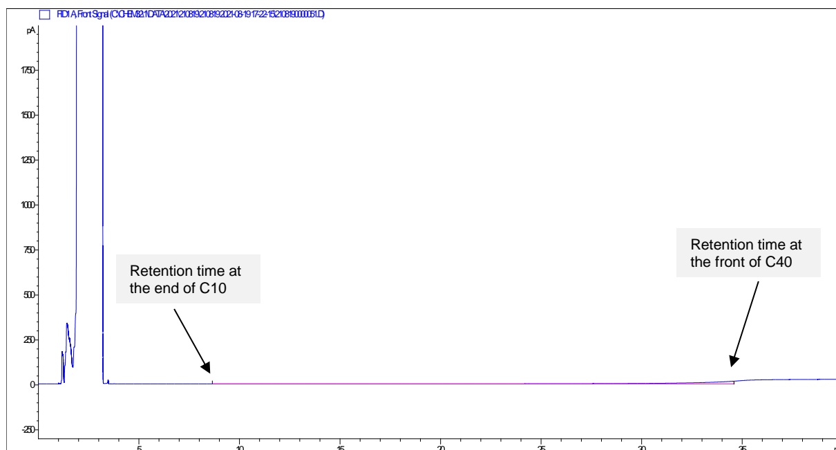
Fig. 3: Integrated GC-FID chromatogram of n-heptane (blank, pure solvent used to prepare BAM-K009a solutions) between the retention times of C 10 and C 40 (analyzed on a BPX-5 column)
